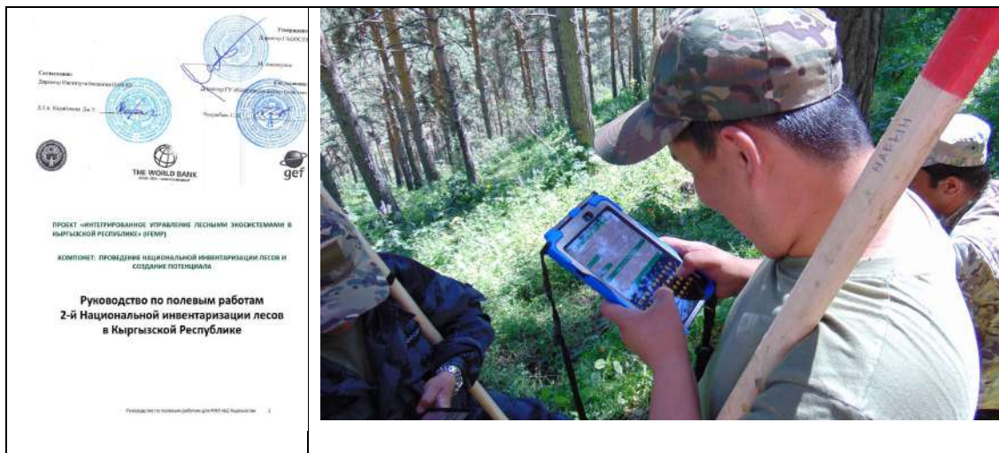
Figure 4-2: For the field data assessment described in the Field Manual modern mobile tablets, GPS and Vertex 6 Geo-Laser devices had been foreseen and successfully used.
